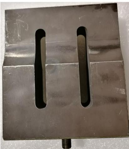
Size: 110 \* 20/15 20K / 2KW, suitable for KN95
