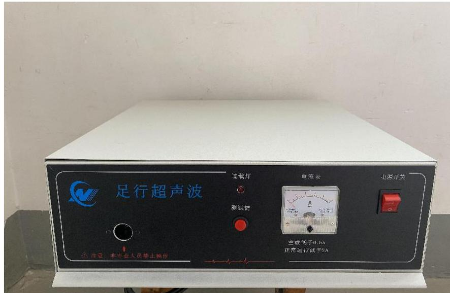
Leveling inductance: adjust the ultrasonic frequency, can not be used to increase power. (Note: Non-professionals are prohibited to operate) Overload lamp: The overload lamp will be on when the pressure is too high during operation. Test key: used in conjunction with the ammeter to test whether the ultrasonic wave is operating normally. Ammeter: start-up surge current 20A, normal operating parameters 0.5A-2A. Power switch: control the switch on and off of the whole ultrasonic wave.
