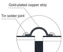
width of the gold belt is less than the width of the b, the use of gold belt/wire bonding interconnect microstrip circuit, no multiple bonding is allowed, the bonding quality should meet the requirements of GJB548B method 2017.1 Article 3.1.5, the bonding strength should meet the requirements of GJB548B method 2011.1 and 2023.2.
